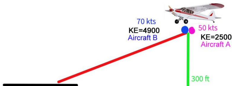
Figure 1. Aircraft A at 300 ft AGL and 50 kts. Aircraft B at same altitude and 70 kts has almost double the kinetic energy assuming same weights.
