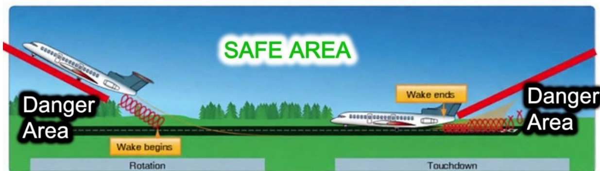
Figure 5-14. Avoid turbulence from another aircraft.
